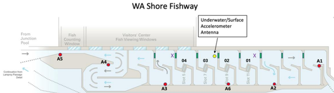
Figure 1. Proposed location of the primary radio tag antenna (depicted by a yellow circle). The two purple Xs are the two additional antenna locations being requested.
