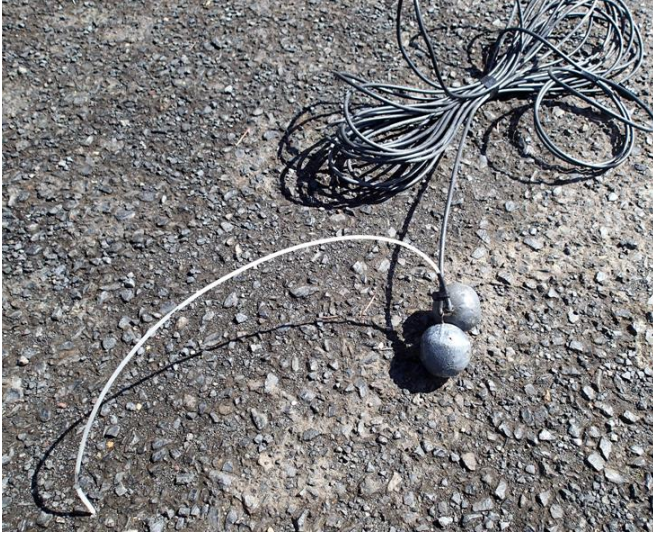
Figure 2. Coaxial cable and weight for an underwater antenna.
